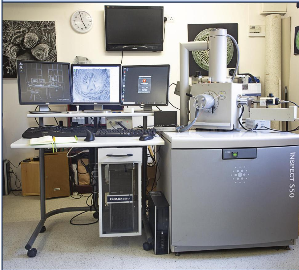
Fig. 1: The SEM as it was at the end of 2019. The right hand screen is connected to the small PC on the floor between the SEM and the control desk and is used to operate the Backscattered Electron Detector protruding from the right of the chamber.
