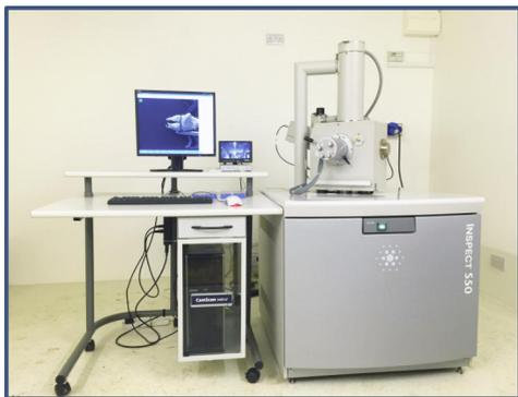
Fig. 2: The SEM following commissioning, in an empty lab - Feb. 2016.
