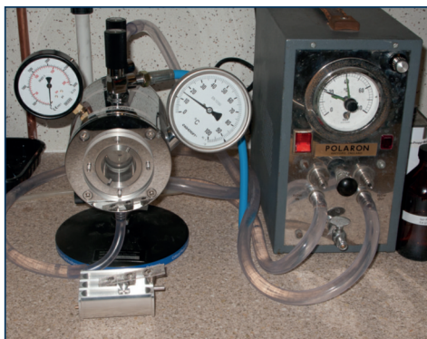
Fig. 3: The Critical Point Dryer, on left, with its boat and mesh basket on the bench in front. The instrument on the right is for circulating warm water round the water jacket of the dryer.
