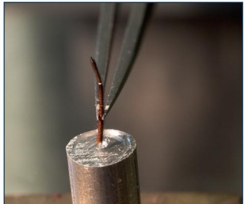
Fig. 3: The leg supported just above the hole in the rod, prior to being lowered into position
