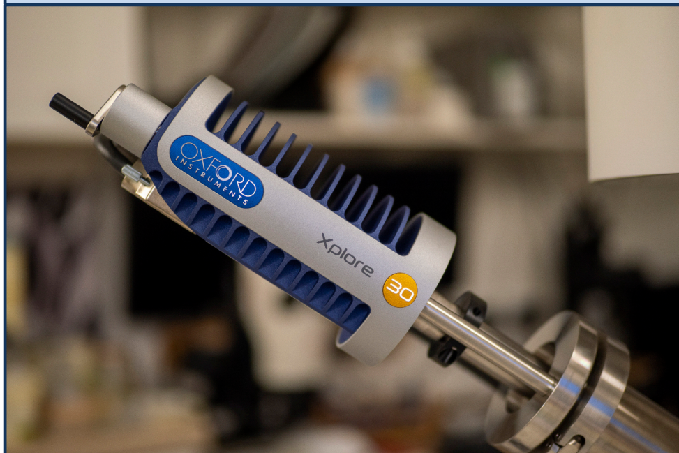
Fig. 1: The sensor for the new EDS system, projecting from the side of the SEM chamber
