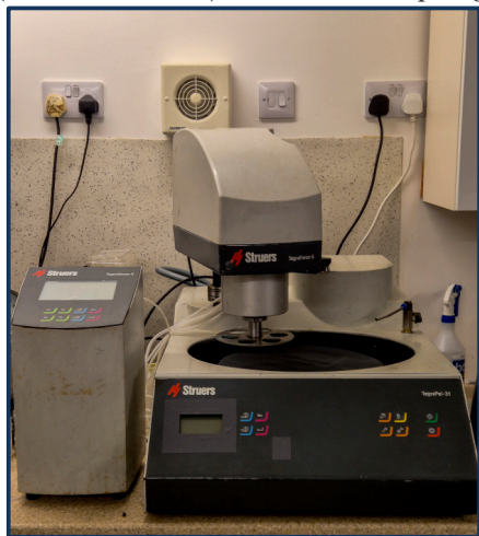
Fig. 5: The replacement polisher. The unit on the left is the doser for providing measured volumes of diamond suspension.
