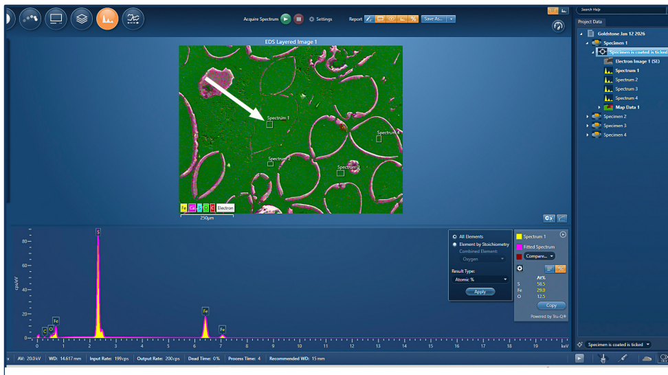
Fig. 2: A screen from the Oxford Instruments EDS software (AztecOne) showing the analysis of the iron pyrites layer of the Goldstone specimen.
