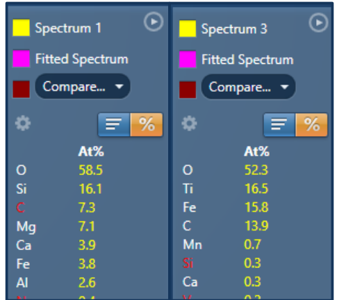
Fig. 8: Showing analysis at two locations. Spectrum 1 is high in silicon and oxygen, suggesting a high silica content. This could be remnants of sand used for casting. Spectrum 3 has a similar amount of oxygen, but no silicon. It also contains metals, namely iron and, interestingly, some titanium. The current best guess for the composition of this area is ilmenite.
