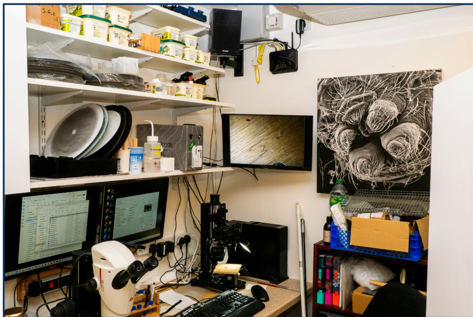
Fig 4: The shelves above the (currently tidy) optical microscopy desk. Note the relocated speaker and monitor. The sloping discs (centre left) are for holding abrasives for the polisher used to prepare rock samples for analysis.
