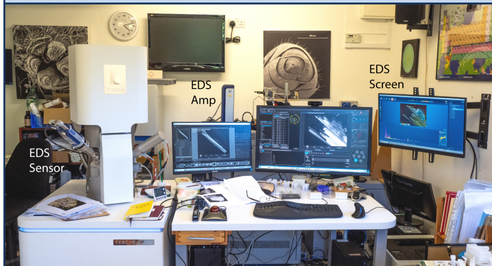
Fig. 1: My SEM on a “normal” working day. Note the new EDS sensor, and also the amplifier (centre) and screen (on the right). The main screen is displaying the SEM User Interface and the screen on the left is displaying a previously captured SEM image. Note also the two canvas prints on the back wall.
